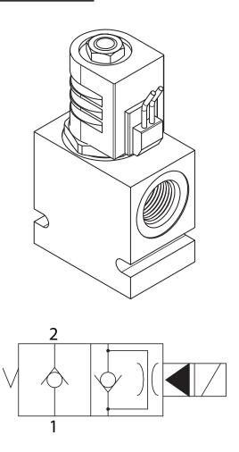
**Normally Closed:** When de-energized the valve blocks flow from (1) to (2) and allows reverse flow from (2) to (1). When energized the valve allows flow from (1) to (2) and restricts flow from (2) to (1).
