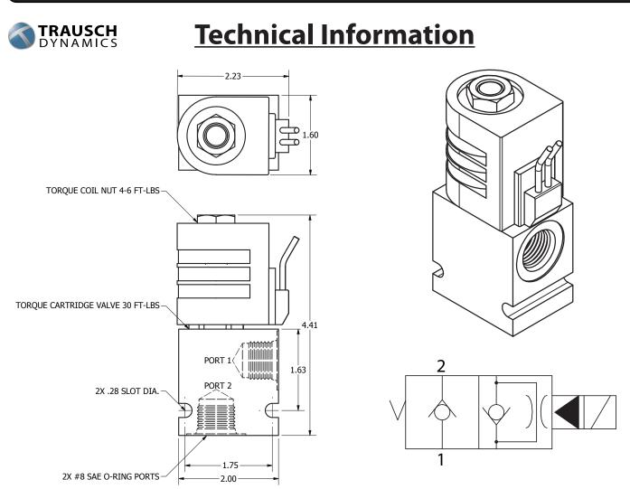
**Normally Closed:** When de-energized the valve blocks flow from (1) to (2) and allows reverse flow from (2) to (1). When energized the valve allows flow from (1) to (2) and restricts flow from (2) to (1).
