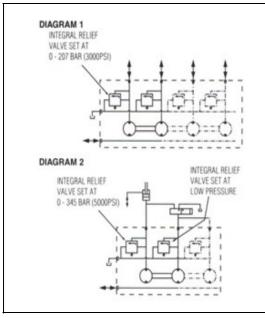
Rotary Flow Dividers split the input flow from a single supply into 2 or more outputs of equal or unequal flows.
