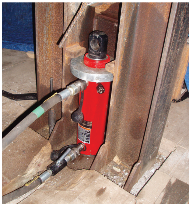
HD cylinders can be used in pushing and pulling applications. In this photo, we see a HD2506 HD cylinder set up for a pull application using a Rod Clevis cylinder accessory
