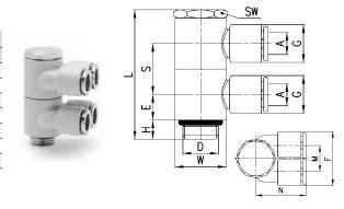
Series 7000 push-in composite fittings are compact and lightweight. They offer easy maintenance of the collet and internal o-ring seal. All materials can be easily recycled.
