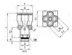
Series 7000 push-in composite fittings are compact and lightweight. They offer easy maintenance of the collet and internal o-ring seal. All materials can be easily recycled.
