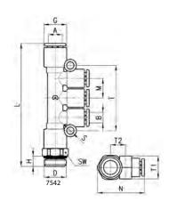
Series 7000 push-in composite fittings are compact and lightweight. They offer easy maintenance of the collet and internal o-ring seal. All materials can be easily recycled.
