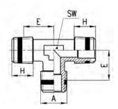
When involved in factory maintenance or plant installation it is often difficult to be absolutely certain which size of fittings will be required. Pipe fittings provide a cost effective solution to this problem. The full range includes straight, L-shaped, T-shaped and cross piece male or female couplings and are available in a variety of thread sizes up to 3/4".
