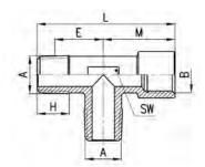
When involved in factory maintenance or plant installation it is often difficult to be absolutely certain which size of fittings will be required. Pipe fittings provide a cost effective solution to this problem. The full range includes straight, L-shaped, T-shaped and cross piece male or female couplings and are available in a variety of thread sizes up to 3/4".
