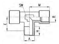
When involved in factory maintenance or plant installation it is often difficult to be absolutely certain which size of fittings will be required. Pipe fittings provide a cost effective solution to this problem. The full range includes straight, L-shaped, T-shaped and cross piece male or female couplings and are available in a variety of thread sizes up to 3/4".
