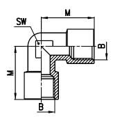
When involved in factory maintenance or plant installation it is often difficult to be absolutely certain which size of fittings will be required. Pipe fittings provide a cost effective solution to this problem. The full range includes straight, L-shaped, T-shaped and cross piece male or female couplings and are available in a variety of thread sizes up to 3/4".
