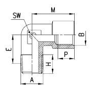
When involved in factory maintenance or plant installation it is often difficult to be absolutely certain which size of fittings will be required. Pipe fittings provide a cost effective solution to this problem. The full range includes straight, L-shaped, T-shaped and cross piece male or female couplings and are available in a variety of thread sizes up to 3/4".
