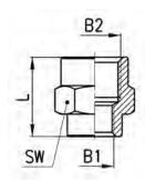
When involved in factory maintenance or plant installation it is often difficult to be absolutely certain which size of fittings will be required. Pipe fittings provide a cost effective solution to this problem. The full range includes straight, L-shaped, T-shaped and cross piece male or female couplings and are available in a variety of thread sizes up to 3/4".
