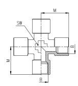
When involved in factory maintenance or plant installation it is often difficult to be absolutely certain which size of fittings will be required. Pipe fittings provide a cost effective solution to this problem. The full range includes straight, L-shaped, T-shaped and cross piece male or female couplings and are available in a variety of thread sizes up to 3/4".
