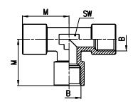
When involved in factory maintenance or plant installation it is often difficult to be absolutely certain which size of fittings will be required. Pipe fittings provide a cost effective solution to this problem. The full range includes straight, L-shaped, T-shaped and cross piece male or female couplings and are available in a variety of thread sizes up to 3/4".
