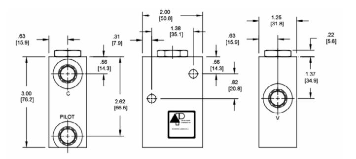
SAE PORTS SHOWN MTG. HOLES ARE .28 DIA. O-RINGS ARE STANDARD ON PISTON ASSEMBLY CHECK VALVE USED IS A PB-CVC
