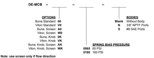
Note: pressure above SPRING BIAS PRESSURE at port (2) may cause valve to self open.
