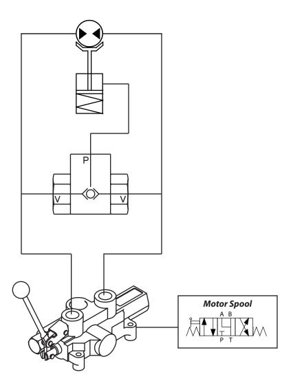
The valve is commonly used to direct oil from the pressure side of a bidirectional hydraulic motor to a pressure-released hydraulic brake. When using this valve as shown above, an A&B-to-tank spool (motor spool) must be used so that the motor brake can drain when the valve is centered.
