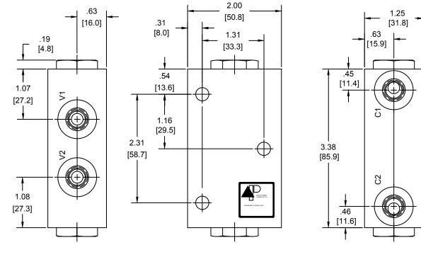
SAE PORTS SHOWN MTG. HOLES ARE .28 DIA. NOTE: DIMENSIONS IN BRACKETS ARE MILLIMETERS O-RINGS ARE STANDARD ON PISTON ASSEMBLY CHECK VALVE USED IS A MA-CVA
