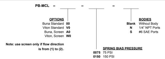
Note: pressure above SPRING BIAS PRESSURE at port (2) may cause valve to self open.
