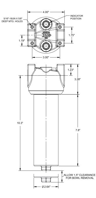
Flows Up To: 30 GPM (114 L/Min) Port Size: 1 1/16"-12 UN (SAE-12) Operating Pressure: 3,000 PSI (207 BAR) Application: Inline Filtration
