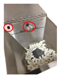
To load the hopper box, lift the lid and pour the Ultra Clean projectiles into the hopper. When filling the hopper, assure that the amount of projectiles does not exceed the Max Fill line shown on the inside of the box. Make sure the ionized air hose and the lid sensor are not obstructed. When ready to operate the UC-CAL, close the lid to the hopper box. The lid of the hopper box should close completely without any added force.
