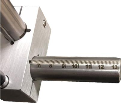
The Marking System comes equipped with laser etched rulers on both the X Axis Rod and Y Axis Rod in metric and nominal inch. To switch between the two, remove the set screw found on the base mount and remove the rod. Orient to the desired ruler and reinsert into the mount. Secure the rod back into position by re-installing the set screw.
