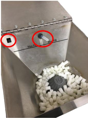
To load the hopper box, lift the lid and pour the Ultra Clean projectiles into the hopper. When filling the hopper, assure that the amount of projectiles does not exceed the Max Fill line shown on the inside of the box. Make sure the ionized air hose and the lid sensor are not obstructed. When ready to operate the UC-CAL, close the lid to the hopper box. The lid of the hopper box should close completely without any added force.
