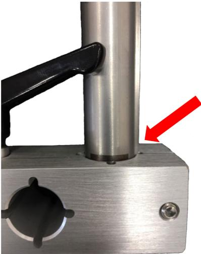
The Y Axis Rod is etched with a reference mark. When changing the rod's orientation, be sure the reference mark is flush with the top of the mount before securing. This assures your logged measurements will remain accurate.
