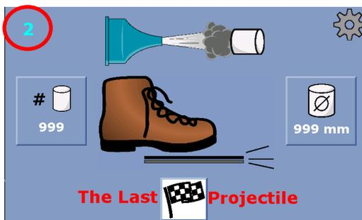
Follow the same prompts as the “**Air Purge +1 Projectile**” cleaning mode. There will be an additional prompt to fire a second projectile. The number at the upper left corner of the screen designated 1<sup>st</sup> & 2<sup>nd</sup> projectile. At the end of the sequence you will return to the air-purge screen to restart the cleaning sequence again. The cleaning procedure is completed when the projectile is verified.
