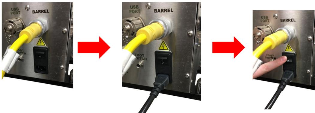
Once you have all of your peripherals connected and the power supply engaged, you may then power on the HMI screen by pressing the rocker switch into the “on” position.
