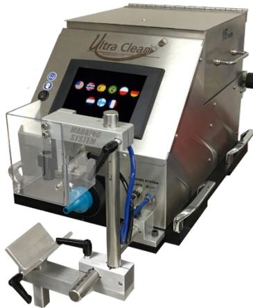
The UC-CAL-MS variant may be equipped with a Marking System. This system is designed to assist the operator with applying a reference mark on their hose during the cleaning process. The reference mark serves as a quality assurance protocol by allowing the operator to visually confirm they have installed a hose fitting to the proper depth during stem insertion.
