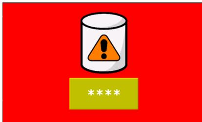
If there is a fault, the system will prompt you to enter a password to clear it. This is to ensure that the operator identifies the issue before overriding the system. Once the issue has been identified and corrected, the password can be entered to resume normal operation.
