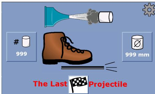
Press and release the foot switch of the UC-CAL Carousel AutoLoader or by activating the trigger of your UC-CAL-HH Hand Held launcher. [Activation occurs upon release of foot pedal or trigger]. The cleaning procedure is completed when the projectile is verified. After Projectile Verification, the next projectile will automatically be loaded.
