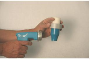
3. Connect supplied UC-QRC-C to a  $\frac{1}{2}$ "ID air hose to launcher and insert nozzle into hose, tube or pipe.
