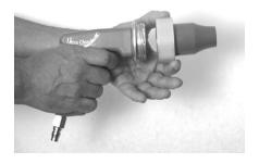
2. Load projectile into nozzle and screw locking ring onto firing head.
