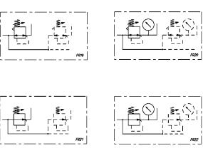
FR19 = Manifold regulator with relieving and without manometer FR20 = Manifold regulator with relieving and manometer FR21 = Manifold regulator without relieving nor manometer
