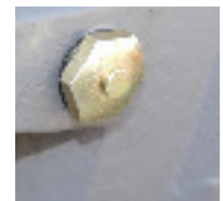
Grease pressure reliefs act to battle overgreasing
