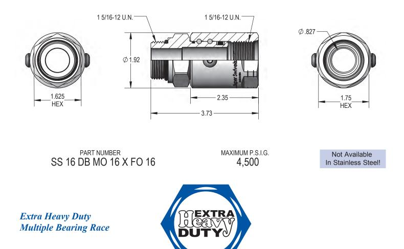
For extreme duty applications **Extra Heavy Duty** swivel offer a multiple bearing race design for superior side load strength and added load bearing support.
