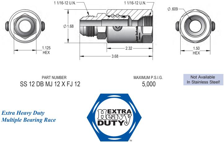
For extreme duty applications **Extra Heavy Duty** swivel offer a multiple bearing race design for superior side load strength and added load bearing support.
