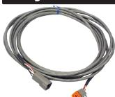
• Use these harnesses to extend the length from your switch box to your valve assembly • Shielded wire • 18 gauge wires • **IP69 Deutsch Connectors**
