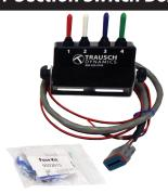
• 4.70" x 1.40" x 2.80" black switch box • Switch box features easily adjustable bail mount • Heavy duty 10 Amp Switch • Momentary switches (on)-off-(on) • Long bat handle switch for easy actuation • Switches are color coded • 3' wiring harness • 6' power cable • Shielded wire • 18 gauge wires • IP 69 Deutsch Connectors • 10 Amp fuse kit • Fuse kit includes instruction sheet
